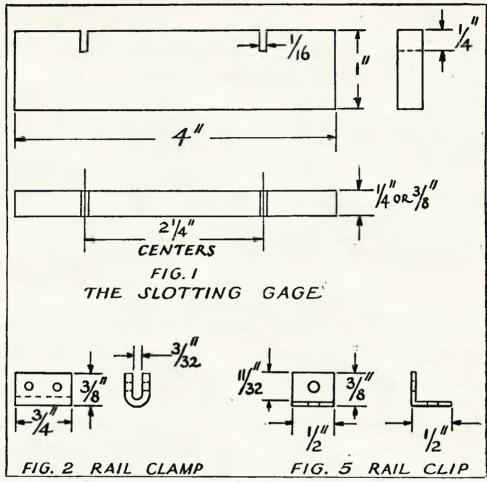
(Fig. 1) The Slotting Gage Is Made From  $1" \times 1/4"$  or 36" Rolled Steel. (Fig. 2) For the Rail Clamp Use  $3/4" \times 3/32"$  Soft Steel. Drill and Tap for No. 6 32-Thread Machine Screw 1/4" Long. (Fig. 5) Material for the Rail Clip Is 1/32" Soft Steel or Brass 1/2" Wide Bent as Shown. Solder or Bolt to Rail. If Bolted, Drill as Indicated, Using 9/64" Drill for No. 6 32-Thread Machine Screw. Attach to the Tie With  $1/16" \times 3/8"$  Wood Screw
